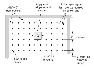
3 LOWER PAN into position. Make sure it aligns with line drawn in Step 1. Avoid stepping on pan until adhesive has cured.
